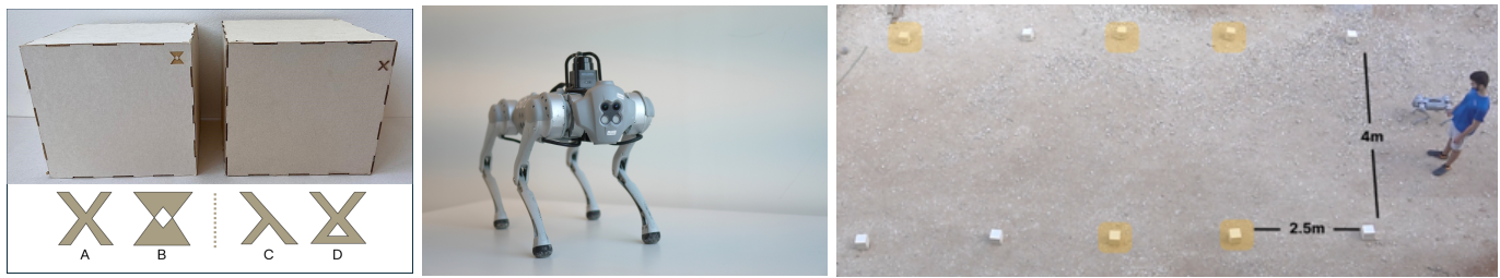
Fig. 2. Left - Cubes and target symbols. A & B are the participants' target symbols; C & D are the robot's target symbols. Center - The unitree Go1 quadruped robot used in the experiment. Right - Organization of the cubes and distances. Cubes with the participant's target symbols are marked in yellow.
