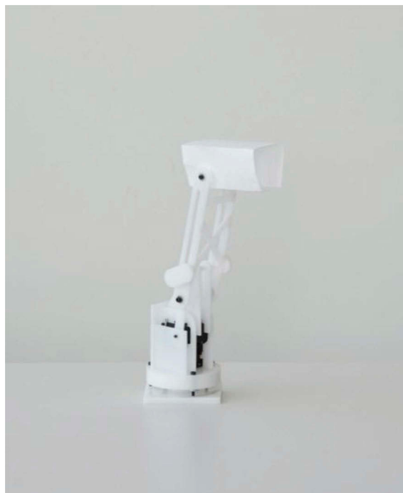
Figure 2. The robotic object used in the study; a 2 degree-of-freedom non-humanoid robot called Kip.
