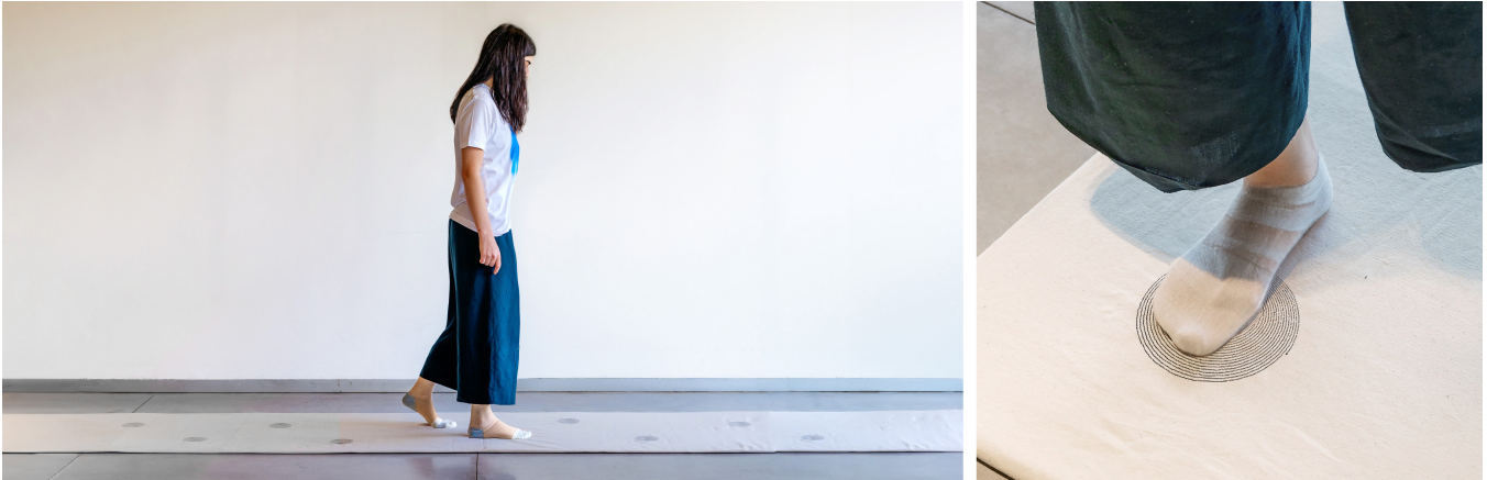
Figure 1: The walking meditation mat, designed to generate feet-focused targeted heat sensation. The mat was evaluated in walking meditation context with two groups, with or without heat, to assess the potential of the heat sensation to guide attention inward.
