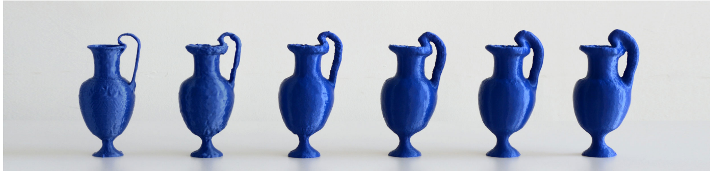
Figure 2: The "chain of digital reproductions", continuous reproduction process increases imperfection and leads to unique aesthetics.
