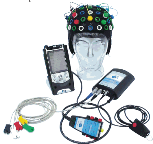
Fig. 2. Components of the BCI system. EEG cap with electrode positions according to the international 10/20 system; EEG amplifier and acquisition unit consisting of g.MOBILab and the Pocket PC; connector boxes to plug in the EEG electrodes.
